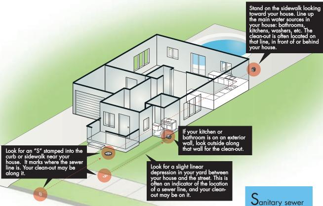
here are a number of places to look for your sanitary sewer clean-out. Start by checking to see if there's an "S" stamped into the concrete of your curb or sidewalk. This marks the location of the sewer line, and your clean-out may be aligned with this marking.
